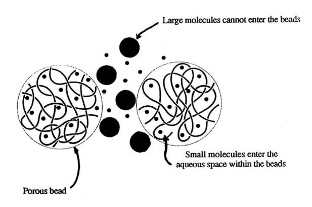
Figure 3.13. An enlargement of the beads and solutes within a gel filtration column.
