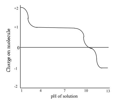
Figure 3.16. Experimentally derived titration curve for lysine. Corresponds to Figure 3.9 in text.
