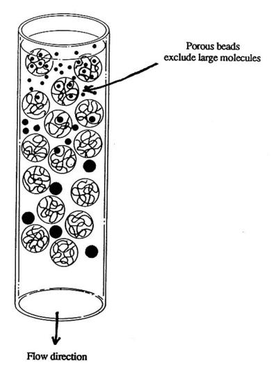
Figure 3.12. A schematic representation of a gel filtration column.
