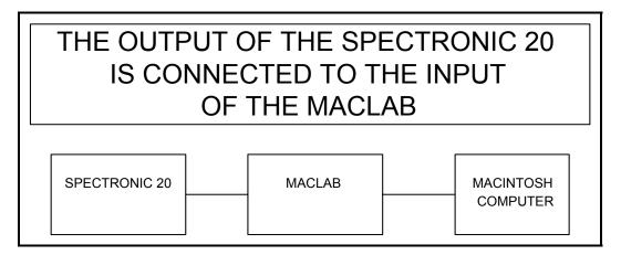
Figure 6.1. Block diagram of the MacLab system used to record transient changes in the turbidity of various blood/solute solutions.
