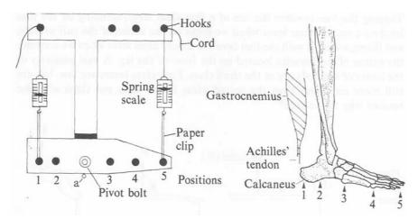
Figure 6.4. A diagram of the kinematic model (left) and the human lower leg and foot (right). An eye-ring is attached at position"a". Positions 1 and 2 represent attachment points for the gastrocnemius muscle, whose contraction produces an inforce on the calcaneus. Positions 3, 4, and 5 represent points on the front of the foot where an out-force can be measured.
