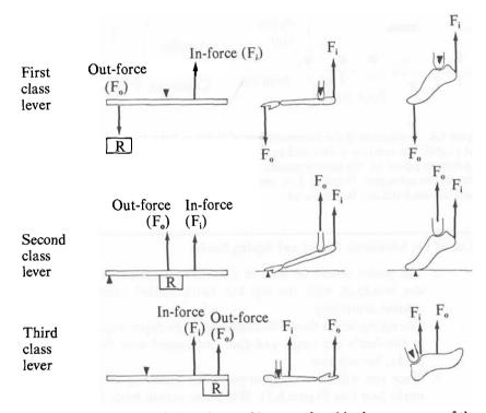
Figure 6.3. Illustration of three classes of levers as found in the movements of the arm and foot. R represents the resistance, against which the out-force is applied and the fulcrum is at  $\triangle$ . (Adapted from M. Hildebrand: Analysis of Vertebrate Structure. Copyright © 1974 by John Wiley and Sons, New York. Reprinted with permission.)
