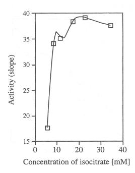
Figure 7B-3. IDH activity is not directly proportional to the amount of substrate added to the reaction mixture.
