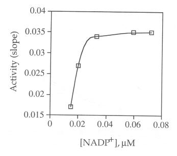
Figure 7C-4. IDH activity is not directly proportional to the amount of coenzyme added to the reaction mixture.
