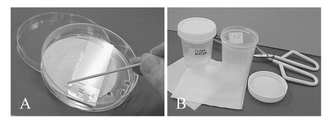
**Figure 4.** A. Scoring along the edge of the membrane-coated collection slide. B. Items to assemble for the field kit. Barbecue tongs may extend your reach in difficult areas!
