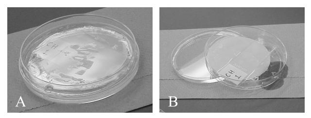
**Figure 3.** A. The dry collodion membrane floating on the water surface above the slide. B. The collodion membrane membrane spread out on the slide and the damp filter paper. It should dry overnight in this position.
