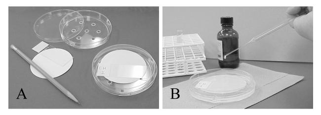
**Figure 2.** A. The petri dish lid and strainer, and the arrangement of filter paper and slide before adding water to the dish. B. Dropping collodion solution onto the water surface above the immersed slide.
