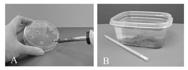
**Figure 1.** A. Melting drain holes in the strainer with a soldering tip. B. A laboratory "environmental" biofilm container with about  $100 \text{ cm}^2$  of surface area.
