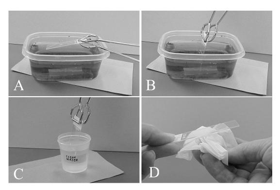
**Figure 5.** A. Horizontal contact of the collodion membrane with the floating biofilm. B. Vertical withdrawal of the slide from the water. C. Vertical immersion and withdrawal of the slide in the rinse water. D. Drying off the back of the slide. Avoid touching the biofilmed side.
