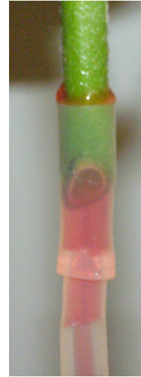
Figure 16. Stem tightly seated in Silastic adapter. Pinch clamp should now be opened.
