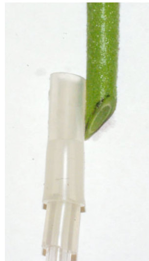
Figure 10. Choosing Silastic adapter size to fit stem snugly. Note 2 nested sizes are needed.
