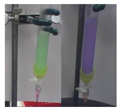
Figure 7. EGFP-Ubx and mCherry-Ubx protein on a Ni-NTA resin column.
