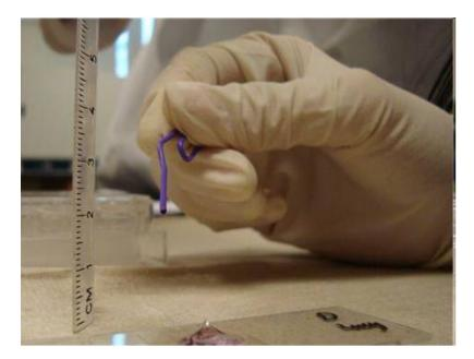
**Figure 8**. Pulling an mCherry-Ubx rope from a slide using a plastic-coated paperclip. Notice the "Hershey kiss" shape at the base that develops from the tension of the rope as it is pulled from the drop.
