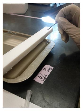
**Figure 9**. Setup for pulling rope from a Teflon coated pan. The pan is filled with Buffer G. Protein is pipetted along the surface of the buffer. The solution is allowed to stand undisturbed for 4 hours to overnight. A Teflon bar (or microcentrifuge rack) is gently placed at the back edge of the pan and dragged forward to within about 2.5 cm of the front edge of the pan. A syringe needle is used to pull the rope.
