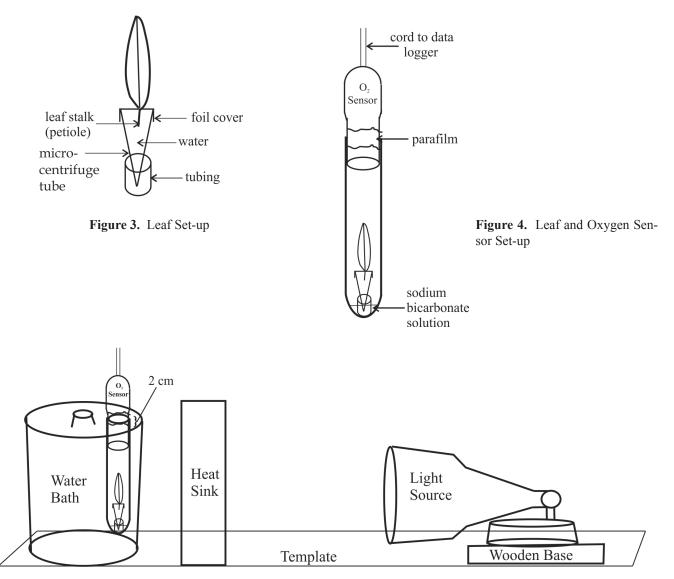
Figure 5. Side View of Experimental Set-up
