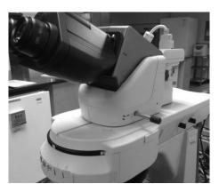
**Figure 4.** Directing light to the camera. When you wish to take a photograph, pull the silver rod at the lower right of the oculars to its outer position as shown.
