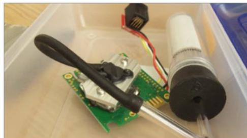
**Figure 11.** Setup in pencil box for direct measurement with the K30 Tube Cap Adaptor.
