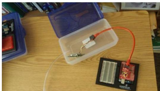
**Figure 12.** Setup to measure yeast. The CO<sub>2</sub> will enter and fill the pencil box and be sensed by the K30 Sensor. The Arduino connected to the K30 Sensor relays the reading to the laptop.
