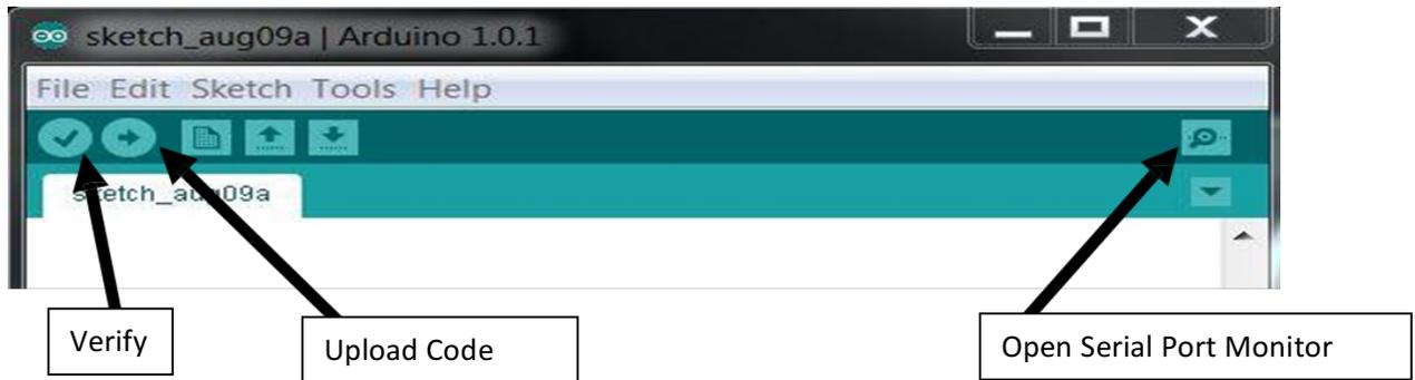
**Figure 19.** Arduino IDE and the indication of where to open a serial window, which is a window that shows the data output in ppm. Once you verify the code, and upload it to the Arduino (The K30 sensor must be attached to the Arduino).
