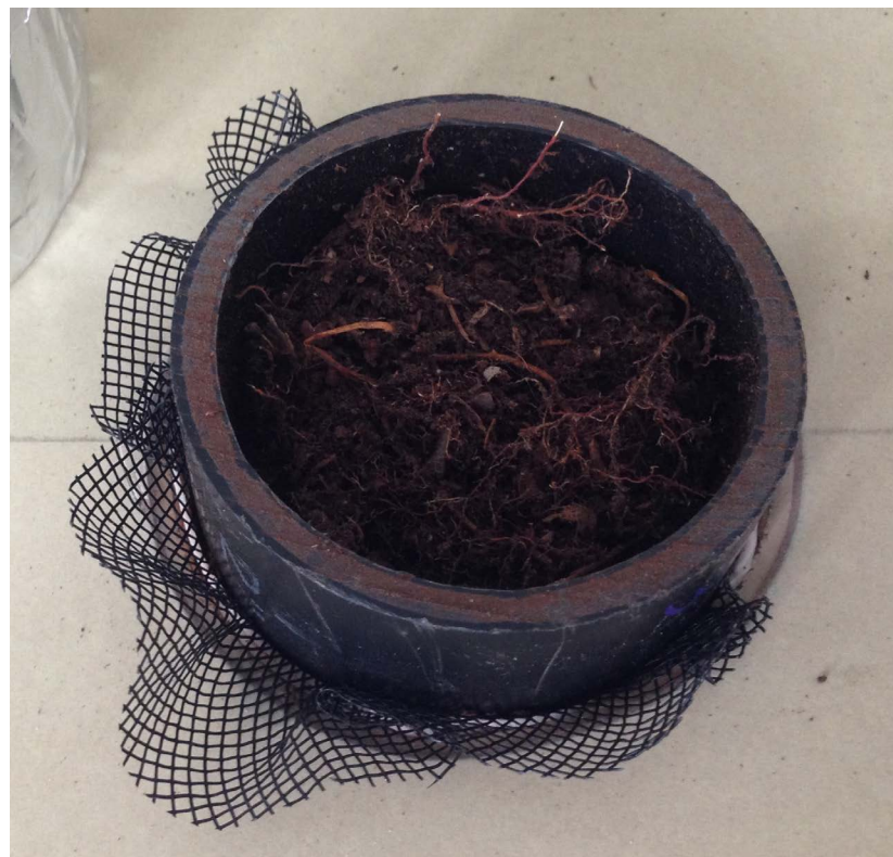
Soil cores were sampled and stored in 5cm X 5 cm PVC pipe pieces. Intact cores are recommended for use in the extractor instead of grab samples as they increase extraction efficiency 1 .
