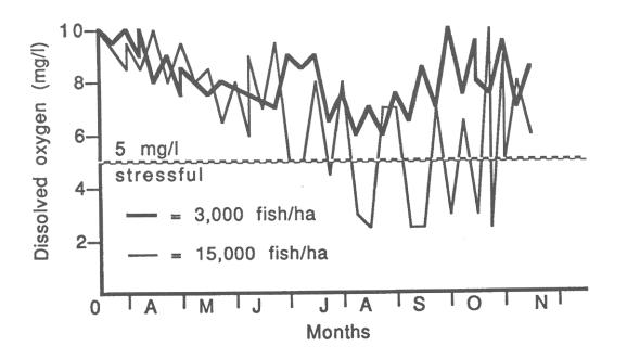
**Figure 10.2.** Dissolved oxygen concentrations in pond simulations containing 3,000 catfish/hectare (dark line) and 15,000 catfish per hectare (light line). No emergency aeration was used in either case. The low oxygen concentrations in the 15,000 fish/hectare case caused 10.6% mortality.
