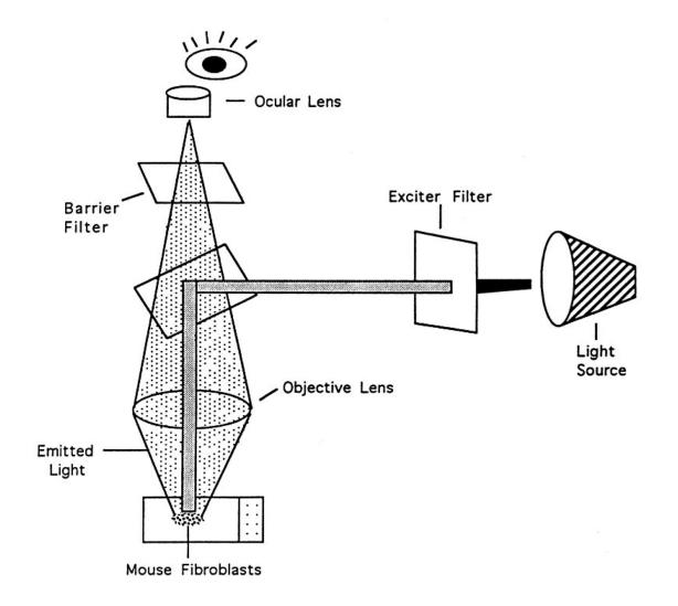
Figure 5.1. The fluorescent microscope
