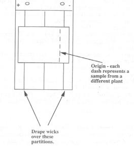
Figure 4.2. Diagram of a cellulose acetate electrophoresis chamber. Pour electrode (running) buffer (Tris-Glycine) into each of the four compartments, but do not let buffer
