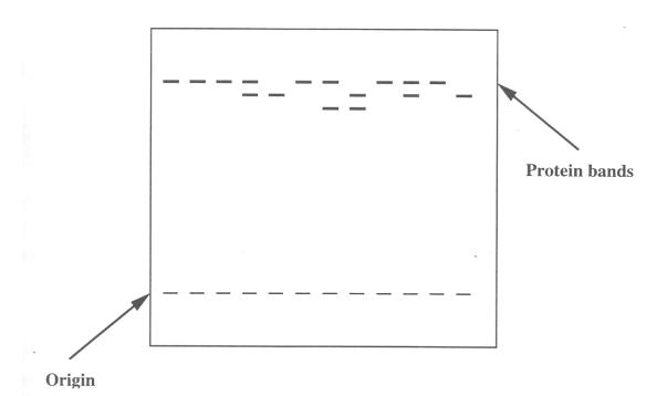
**Figure 5.1. Diagram of a cellulose acetate electrophoresis gel for** <u>*Lap*</u> **in white campion.** Each lane represents protein from one individual. Homozygotes display only one protein band, while heterozygotes display two bands. Protein bands are numbered based on their rates of migration, with the fastest migrating band designated as 1. From left to right, the phenotypes are: 11, 11, 11, 12, 22, 11, 13, 23, 11, 12, 11, 22.
