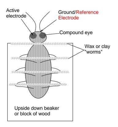
Figure 1. Diagram of electroretinogram set up.
