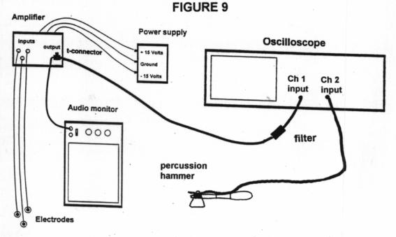
2. Set the oscilloscope sweep speed (<u>SEC/DIV</u>) to 10 msec/div. Press <u>CH2/MENU</u> button until a second trace for Channel 2 is seen on the oscilloscope screen. Adjust Ch2 <u>POSITION</u>, if needed.
