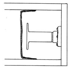
**Figure 18.1B.** Top view, looking down into one end of the inside of the gradient box. This end has the ceramic heating element protected by wire screening.
