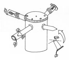
**Figure 19.3**. This bioassay chamber uses four microcentrifuge tubes as replaceable housing for the experimental subjects and substances. Nonwoven polyester caps separate the interior of each tube from the interior of the bioassay chamber. These barriers allow odors and sounds to pass through, but *Melittobia* will remain separated — unless, as occasionally happens, a determined individual chews a hole through it!
