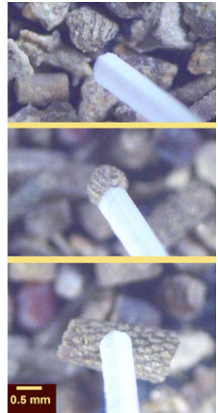
Figure 4. Rubber-tipped widget. The moistened tip of a widget is used to pick up a microfossil from the sorting dish and to transfer it to a water-filled dish. The top panel shows the widget tip as it is held above the granules. The middle panel shows a charophyte oogonium stuck to the wet tip of a widget. The lower panel shows a fragment of bryozoan colony stuck to the tip of the widget.
