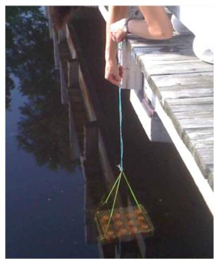
**Figure 3.** Plant pot method in the field. Nutrient containing plant pots are lowered into a pond to test the nutrient deficiency in pond water. Adapted from Bushong & Bachmann (1989).
