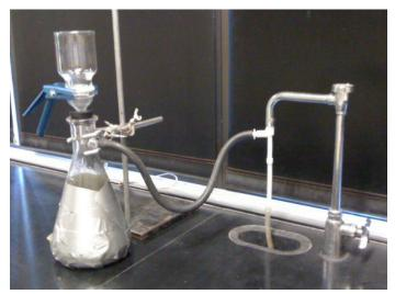
Figure 4. Assembled filtration flask, funnel, filter, and clamp attached to water pump.
