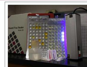
**FIG. 6:** Colilert assay showing sample bottle, reagent packets, Quanti-Trays with positive wells (yellow, coliforms; fluorescent, *E. coli*), Quanti-Tray sealer, and UV lamp.
