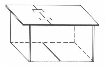
**Figure 8.1.** Plastic cage with hinged plexiglass top for assaying female sex pheromone. A line is drawn on the bottom of the cage to aid in counting the locomotory activity of males stimulated by sex pheromone.
