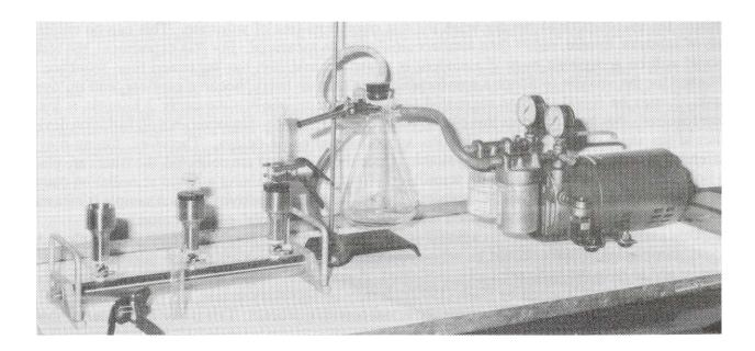
**Figure.9.3.** A workstation suitable for a pair of student is a vacuum manifold with filter units, a filtrate trap, and a vacuum pump; these are standing on absorbent paper in a tray that has a raised edge.
