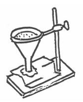
Figure 9.1. One of two equipment set-ups for demonstrating relation of surface area to passage of materials.
