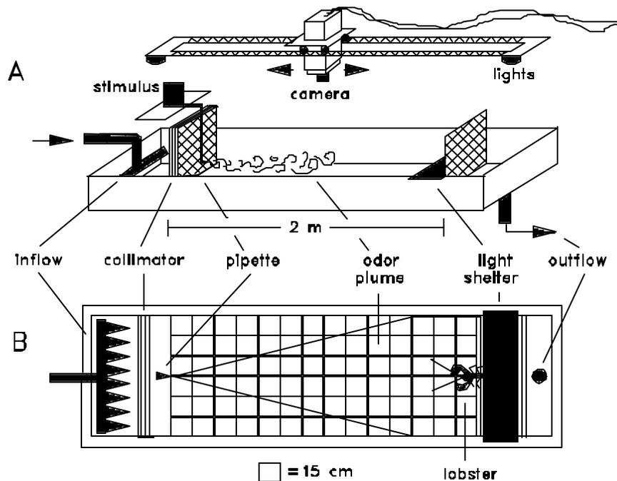
**Figure 12.3.** Side and top view of a flow-through tank (or “flume”) used to study chemically-mediated behavior. The flow-through system is needed to insure that the animal does not habituate to the stimulus. Collimators help produce even flow across the tank, and can be easily constructed from straws or fluorescent light grating. The size of the tank is adapted to the size of the animal, at least four body lengths, but preferably more. (from Moore et al., 1991)
