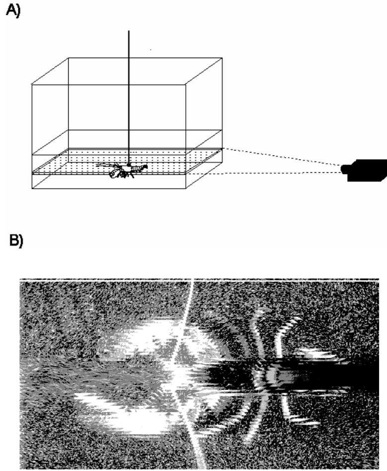
**Figure 12.4.** (A) Diagram of a “no flow” tank used for visualization of animal-generated currents. The size of the tank needs to be large enough to prevent “wall effects”, i.e., distortion of the currents by the aquarium walls. The animal is held in place by a plastic bolt and a rod with a plastic screw. (B) Long exposure photograph of lobster gill current visualized with neutrally-buoyant particles. (Photograph by Thomas Breithaupt and George Gomez)
