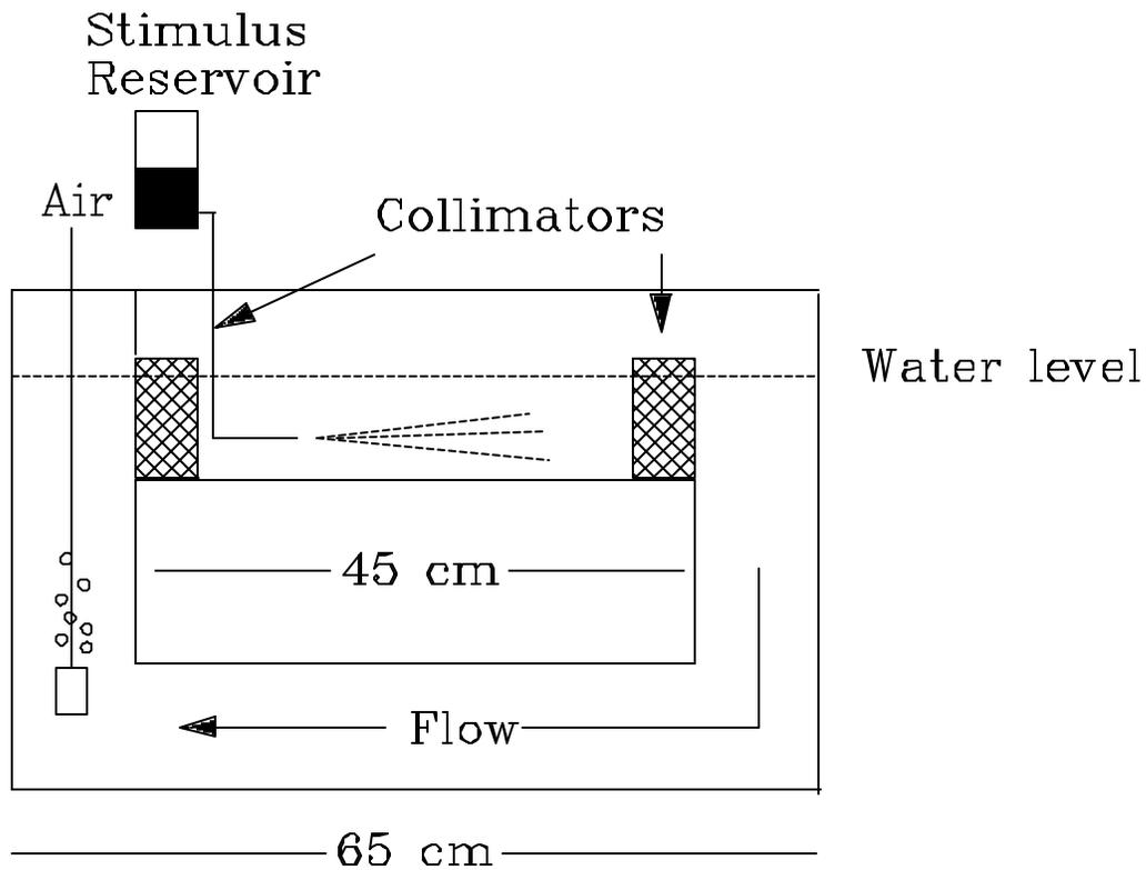
**Figure 12.2.** Diagram of a recirculating flume. The flume can be driven by air or a small propeller. This set-up is preferable for experimentation with marine invertebrates when running seawater is not available. However, eventually, built-up of stimuli will adapt the animal's chemoreceptors and prevent the animal from exhibiting orientation behavior.
