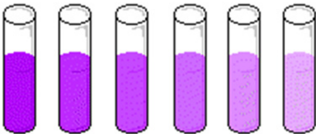
Figure 4. Serial Dilutions - The solution becomes less concentrated in each consecutive round of dilution, demonstrated by the fading purple coloration above. In this process, a solution is successively diluted from a neat (undiluted) sample to form a series of dilutions that each originates from the previous dilution.
