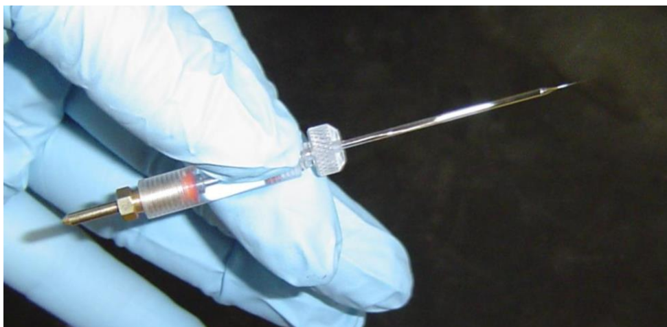
Figure 14: Microelectrode assembly with glass capillary in place.
