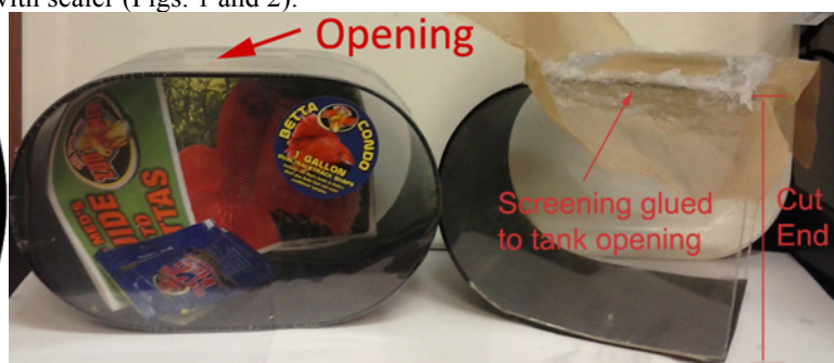
Figure 2. Photo of Beta tank before and after it is cut and prepared for use in larger tank.
