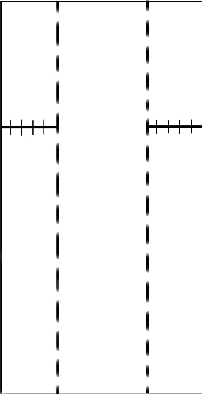
**Figure 1.** This diagram represents (1:1 scale) where cuts should be made on a cardboard rectangle that will become a mirror chamber. Vertical dashed lines indicate where the cardboard should be scored half-way through, and horizontal lines with hatch marks indicate places where the piece of cardboard should be cut all the way through. Sequence of cuts is unimportant.
