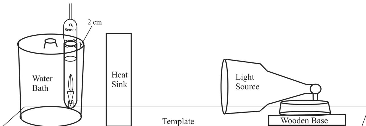
Figure 5. Side View of Experimental Set-up
