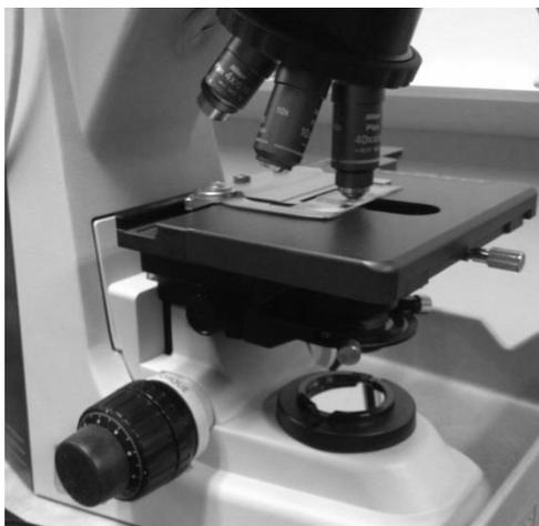
**Figure 3.** Focusing. As you would with any compound light microscope, begin your focusing sequence by lowering the stage and moving the 4X/scan objective lens into position. Start here every time you lose focus or change slides. The stage height (i.e. your focus) is controlled by the focusing wheel on the left side of the scope. The smaller/outer part of the wheel is the fine focus.
