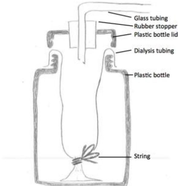
**Figure 1.** Set-up of one model cell. The dialysis tubing is secured at the top by the screw top bottle lid and at the bottom is secured with string. A rubber stopper with glass tubing penetrates the plastic bottle lid.
