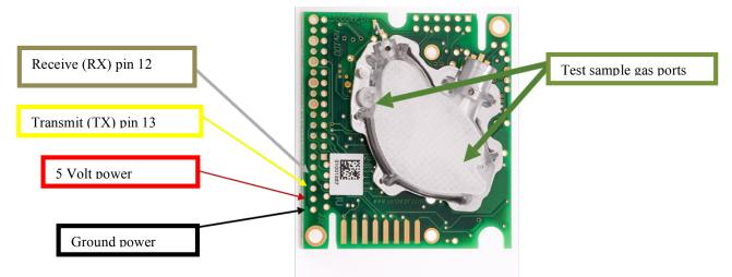
Figure 9. K30 CO2 Sensor (Basic model) and the location of the wire connections.
