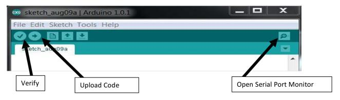
**Figure 19.** Arduino IDE and the indication of where to open a serial window, which is a window that shows the data output in ppm. Once you verify the code, and upload it to the Arduino (The K30 sensor must be attached to the Arduino).
