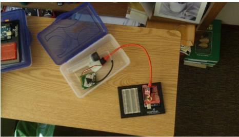
Figure 17. Complete setup for the direct measurement (peas). The germinating peas are loaded into the centrifuge tube, the stopper is replaced, and the box is closed. The  $CO_2$  diffuses from the centrifuge tube into the K30 sensor.
