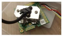
Figure 10. The K30 Tube Cap Adaptor (metal plate with blackturret/nozzle).
