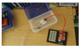
**Figure 12.** Setup to measure yeast. The  $CO_2$  will enter and fill the pencil box and be sensed by the K30 Sensor. The Arduino connected to the K30 Sensor relays the reading to the laptop.
