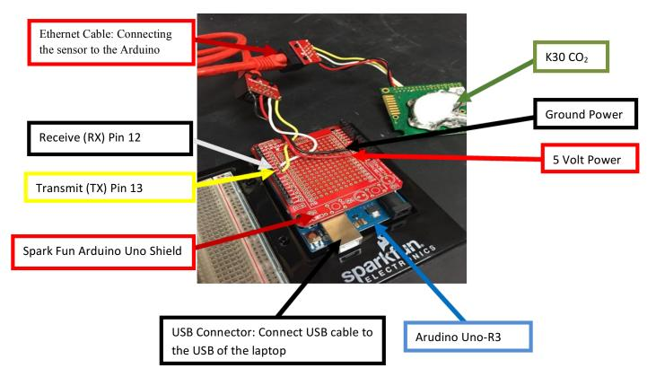
**Figure 18.** Fully assembled K30-Arduino sensing system. Here the K30 sensor could detect the CO2 ppm in the room.
