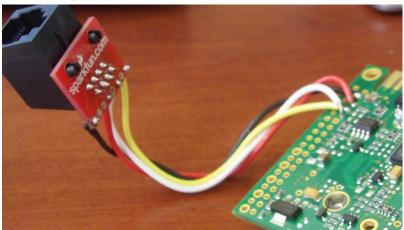
Figure 8. Attaching the assembled RJ45 board to the K30 sensor.
