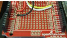
Figure 7. Soldering wire connections to the protoshield (red).
