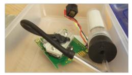
Figure 11. Setup in pencil box for direct measurement with the K30 Tube Cap Adaptor.
