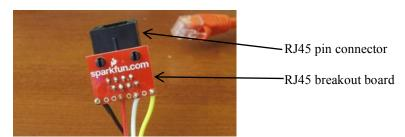
Figure 6. RJ56 Pin connector (black) and RJ45 Breakout Board (red).
